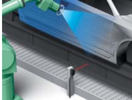
Paint adhered to the sensing surface (Through-beam)
